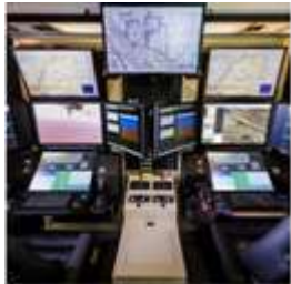
Block 30 Ground Control Station (GCS)
