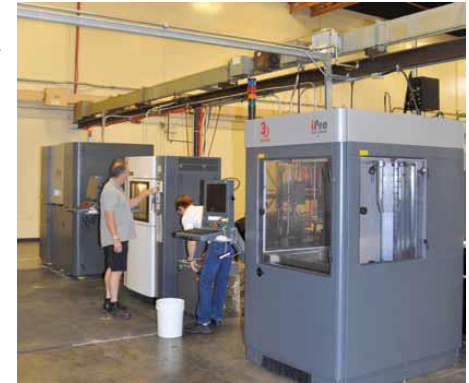
Sheet metal mechanic and reverse engineer program the Fused Deposition Modelling (FDM) 3-D printer. The printer is primarily used to create tooling to aide in the fabrication of sheet metal parts.
