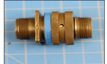
Locked Note- The silver post is visible and a “click” is felt.
