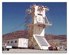
**RDT&E.** Production motors with thrusts up to one million pounds can be heavily instrumented and tested in any of several nozzle-down angles on a one-of-a-kind hydraulic tilt-table, and in the horizontal mode with thrusts to 1.5 million pounds. Developmental or other high-hazard engines with thrusts to 300,000 pounds can also be tested in one of two high-hazard test bays. Additional activities include machining of rocket motors for propellant aging studies.
