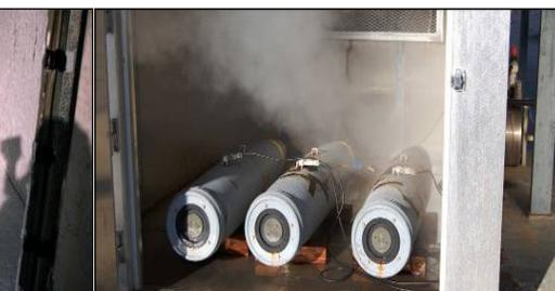
**Climatic. Temperature, Humidity, and Salt-Spray.** Tests are conducted to subject live weapons and their components to simulate natural environments likely to be encountered during the weapon life cycle. Seven temperature controlled ovens are available, the largest being 8 x 12 x 20 feet. Temperatures can be maintained or cycled through any portion of a range of -65 to +180°F. All chambers are temperature and humidity controlled.
