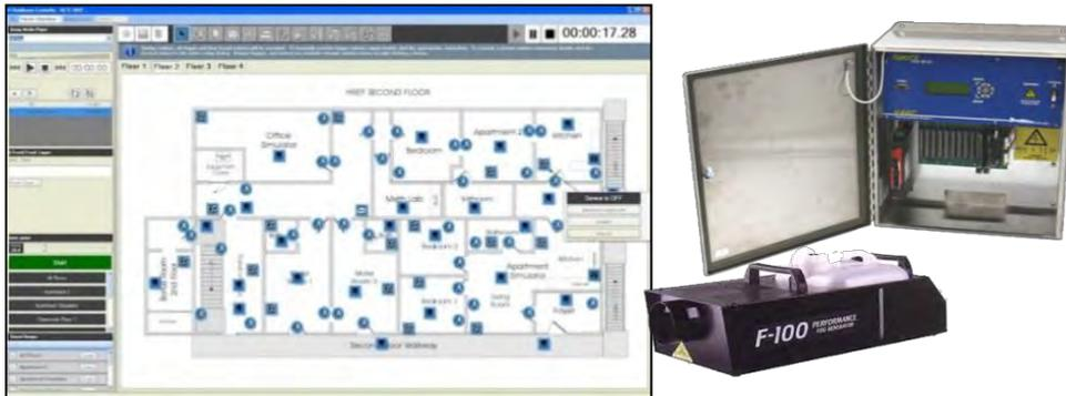
The NAWCTSD Scenario Planning and Effects Control System enables instructor/operators to provide highly detailed and repeatable immersive training scenarios by defining combinations of cause/effect, time, and manual trigger actions between various types of sensor and environmental stimuli for increased training effectiveness, trainee immersion, and reduced instructor/operator workload.
