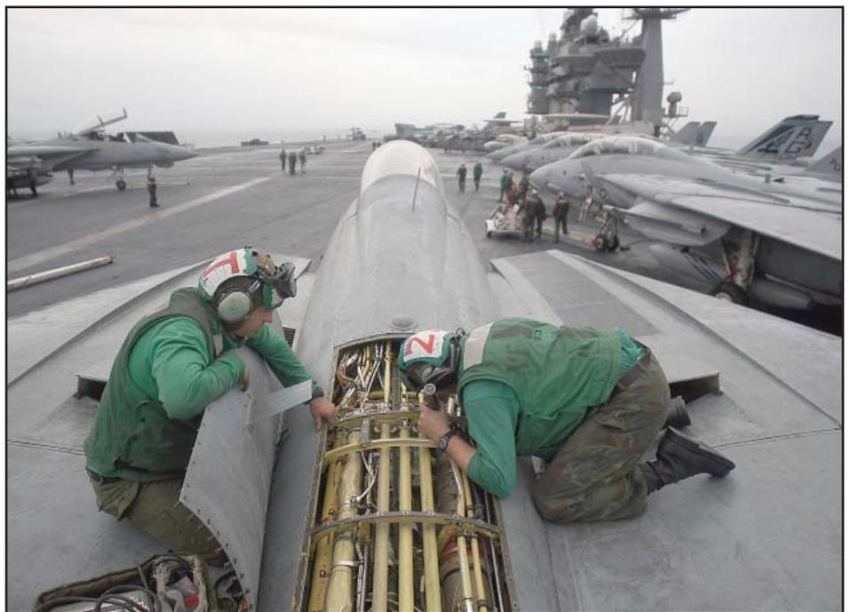
*Sailors perform a wiring inspection on the backbone of an F-14 Tomcat at sea.*
