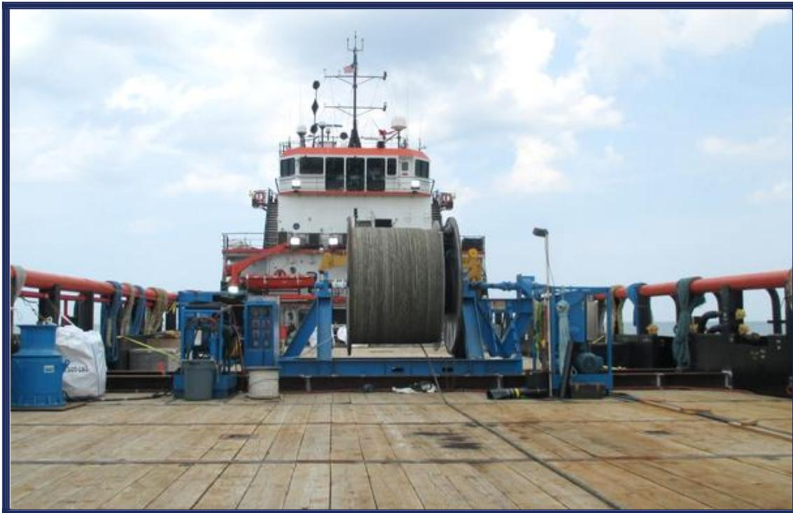
HOS Sweet Water, an offshore support vessel, transfers electro-mechanical-optical(EMO) cable across its deck off the shore of Naval Station Mayport, Florida on July 14, 2015 in support of the Undersea Warfare Training Range (USWTR) program. The USWTR team installed the first 11 kilometers of shallow water EMO cable that will eventually connect the shore-side USWTR system and Range Operations Center to the training range located 50 nautical miles off Naval Station Mayport.(Courtesy photo)
