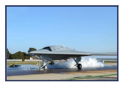
The X-47B prepares for its inaugural catapult shot Nov. 29 at Patuxent River, Md. The Navy's first-ever steam catapult launch of the pilotless X-47B ensures the vehicle can structurally handle the rigors of the unique and stringent aircraft carrier environment. (Photo courtesy of Northrop Grumman)
