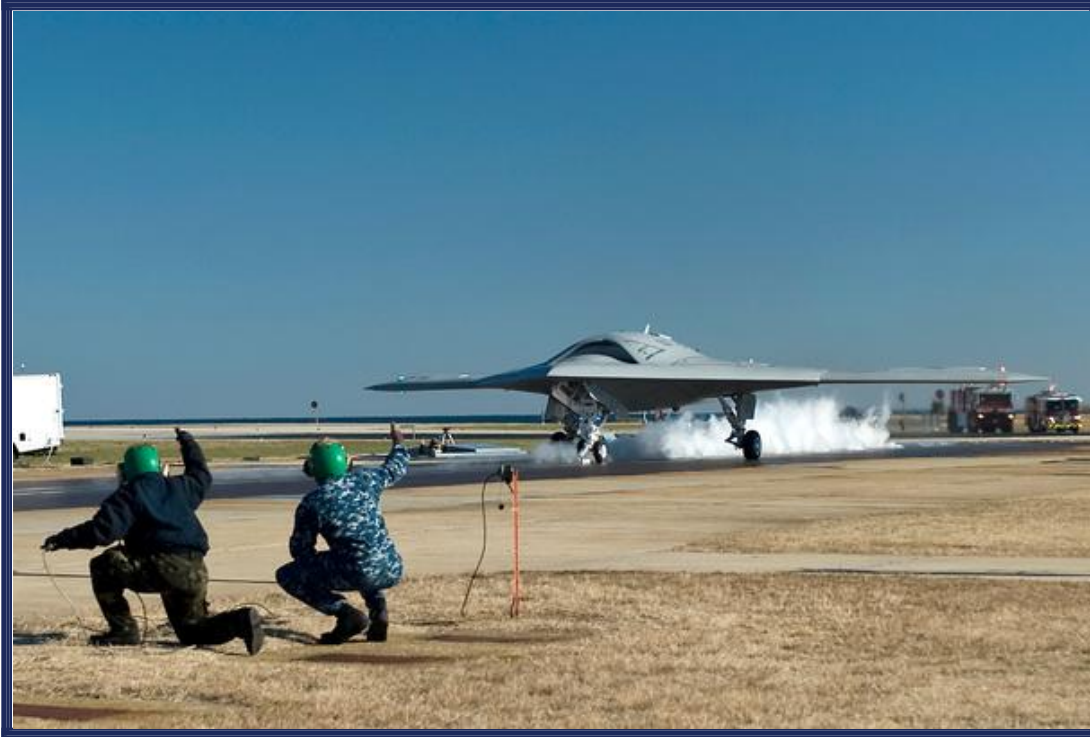
Launching crew prepares the X-47B Unmanned Combat Air System (UCAS) for its first land-based catapult launch Nov. 29 from Patuxent River, Md. (U.S. Navy photo)
