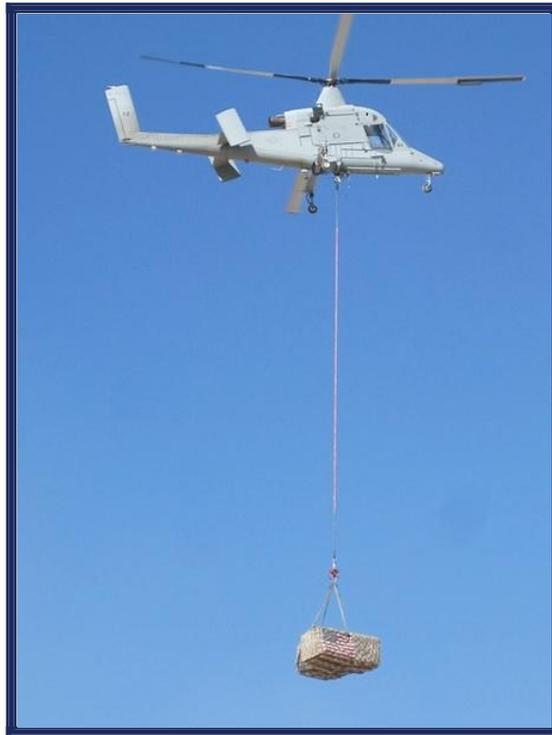
The K-MAX is the Marine's first unmanned helicopter designed for resupplying troops in remote locations. Aviation history was made when Marine Unmanned Aerial Vehicle Squadron 1 operated a K-MAX during its historic 90-minute flight, Dec. 17. Today, the KMAX remains deployed in Afghanistan flying missions operated by Unmanned Aerial Vehicle Squadron 2. (Photo courtesy of Lockheed Martin)
